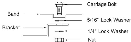
4. Install the band onto the chimney by placing the second carriage bolt through the correct size **square** hole, wrap the band around the chimney, and place the corresponding oval hole over the carriage bolt, and continue to assemble the remaining hardware as shown above. (On smaller diameter chimney the excess band material should be cut off)
