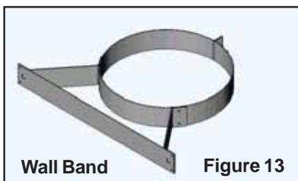
Fasten securely the Wall Band around the chimney with the supplied nut and bolt. Check for clearances and plumb as you fasten the Wall Bands to the wall. Use a level against the chimney section at each support stage to keep the assembly plumb.
