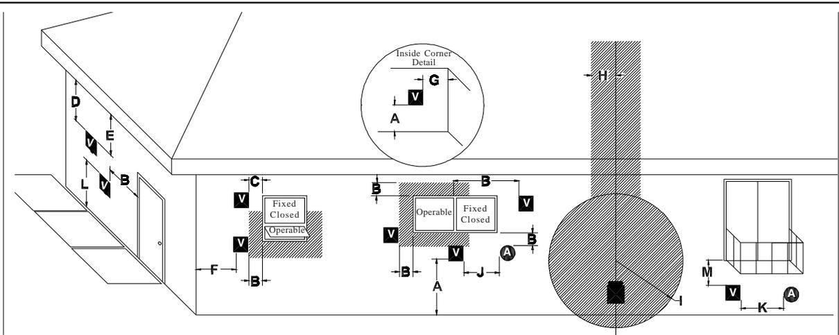
**V** = VENT TERMINAL      **A** = AIR SUPPLY INLET      [Hatched Area] = AREA WHERE TERMINAL IS NOT PERMITTED
